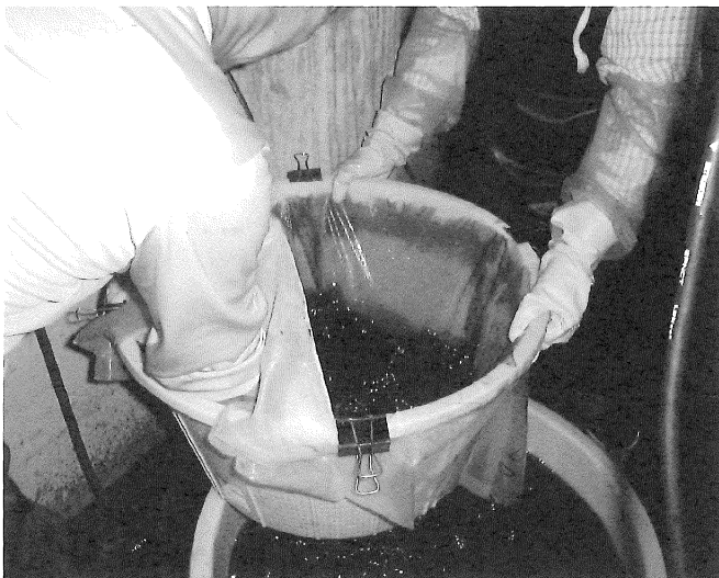
Fig. 3-7. Harvest of M. macrocopa by a plankton net (opening 350 \mu\text{m} ).
